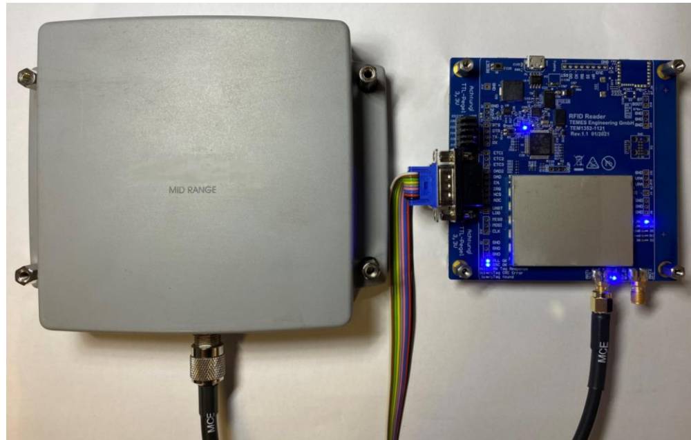
RFID-Board without housing (on the right) connected to a fitting antenna (left)
